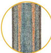
Example of damaged pin plating
