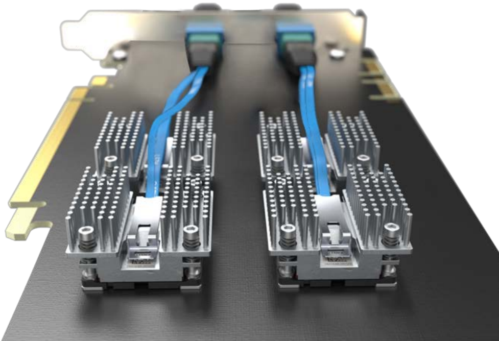
1.2TB PCIe Card Example: Four 300Gb/s optical interfaces with MPO adapter
